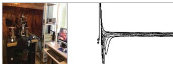
Figure1. patch clamp set up and inward ion currents in neural cells
